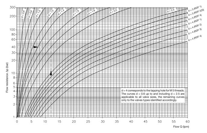
Example: For a gliven flow of 12 lpm a flow resitance of  $\Delta p = 40$  bar is required. The necessary fixed restrictor bore is d = 1.8 mm.
