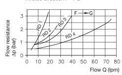
Oil viscosity during test approx. 50 mm<sup>2</sup>/s
