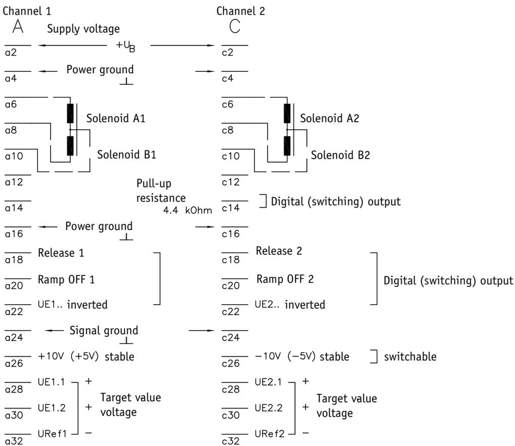
Terminal block according to DIN EN 60603-2
