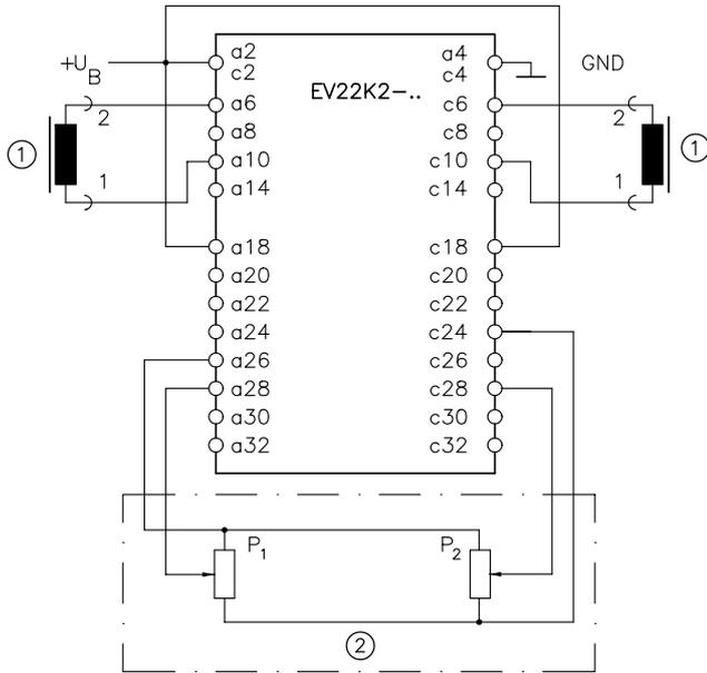
Actuation of hydraulic valves using a proportional solenoid
