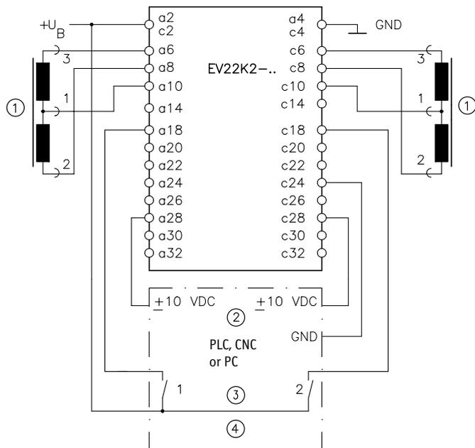
Diagram showing actuation of hydraulic valves with a proportional solenoid
