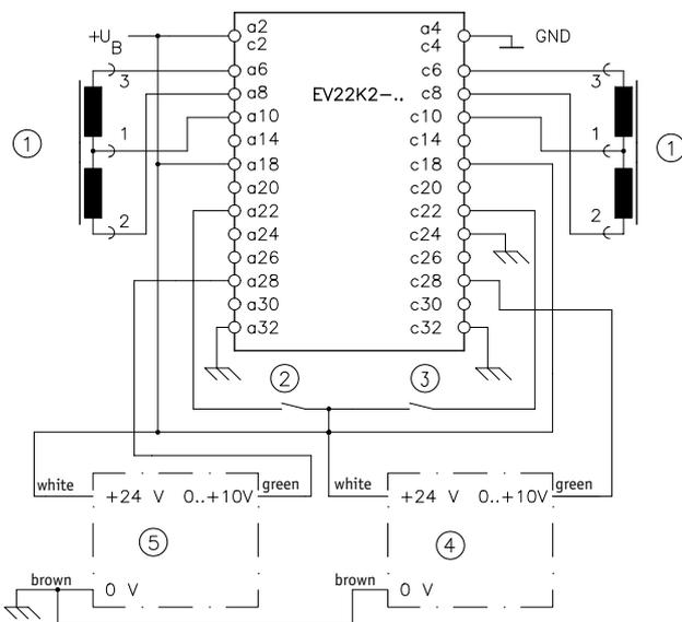
Connection of a joystick switch with active setpoint generator, target value voltage unipolar, e.g.: controller with opto-electronic absolute encoder
