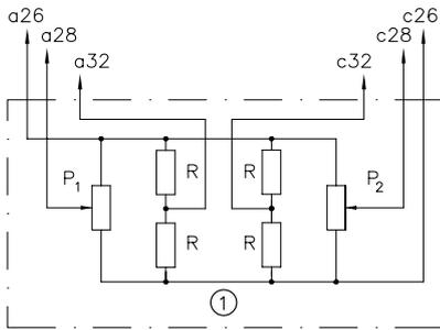
As in example 2, two single potentiometers are used as signal emitters. The target value voltage is bipolar. The absent centre tap of the target value potentiometers is simulated in each case by two additional resistances of the same size between 5 and 10 k $\Omega$ , 0.25 W. This avoids the safety disadvantages of example 2 and the same applies as in example 1.
