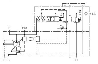
System pressure is tapped within the controller (internal).
