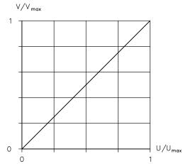
$U/U_{max}$  input signal;  $V/V_{max}$  displacement volume
