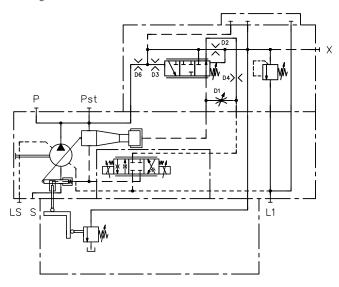
The EM.CH controller can be combined with pressure, LS and/or power controllers to limit pressure and/or power.
